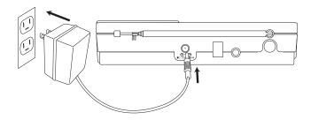
Plug the AC adapter cord into the 12V DC input jack on the back of the unit. Then plug the adapter into the wall outlet. Once plugged in, the internal battery charger will automatically charge the battery if a rechargeable battery is installed, and the "Rechargeable" (RB) setting is selected. Keep the unit plugged in at all times. Then your unit will be ready to use in the event of a power failure.
